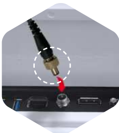
Tighten connection for power
